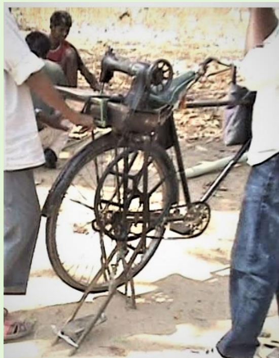
Detail of pedal for Sewing machine
