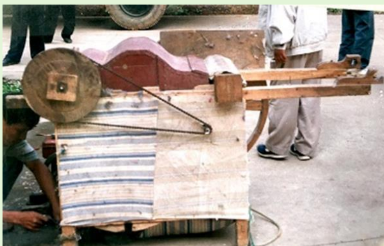
Installing the shredding machine
